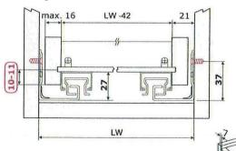
Dimensioni e foratura del cassetto Dimensions and drilling of the drawer 1a(Φ3.5x12)
